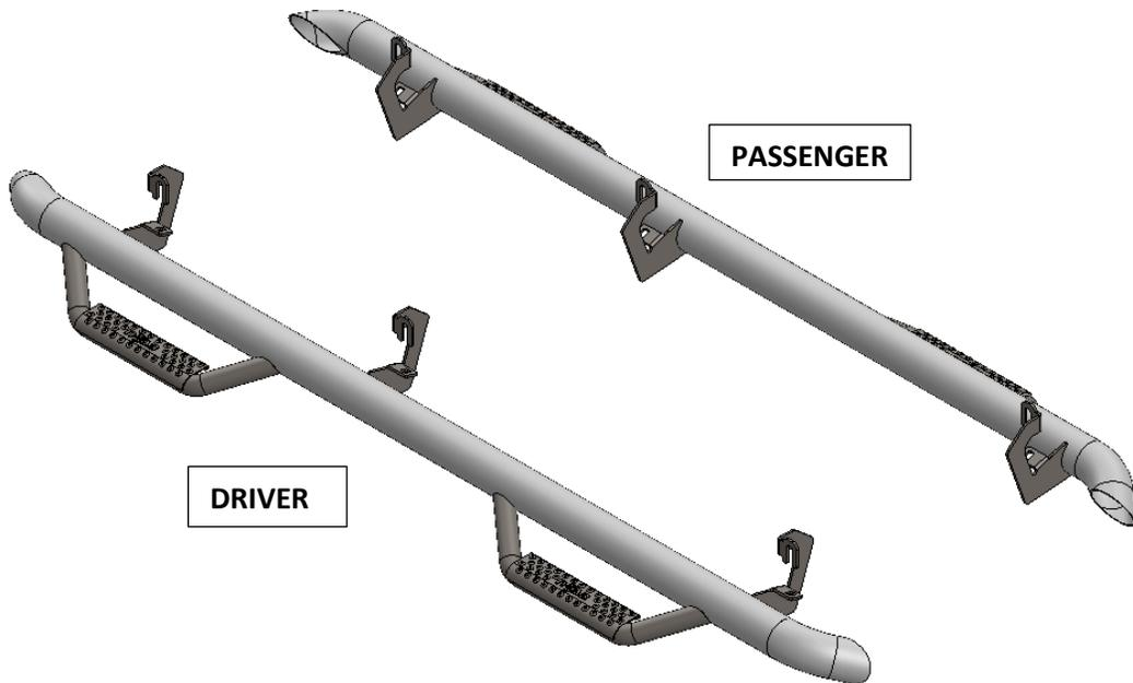
**Step 1:** Starting with the Driver side, Look on the underside of the body and locate the factory supplied mounting positions. **NOTE: Some vehicles require the use of speed clips and nuts, which are supplied with the hardware kit.**
