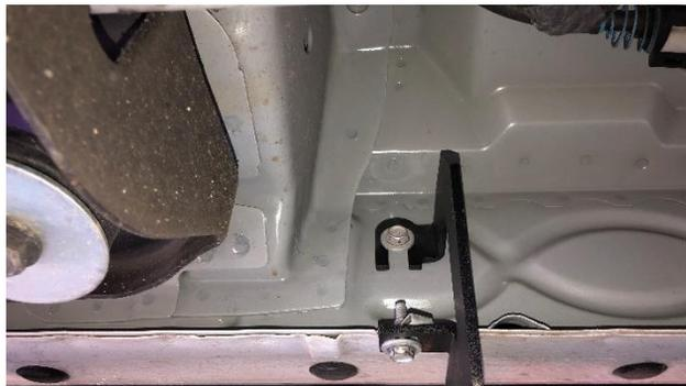
**Step 4:** Next, tighten all hardware beginning with the lower mounts first then the upper mounting locations.
